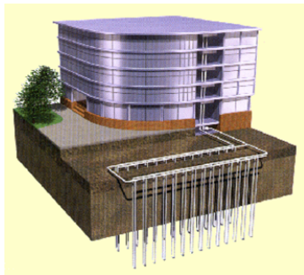
Afb. 9.36 Verticale bodemwarmtewisselaars (bron: GroenHolland)
